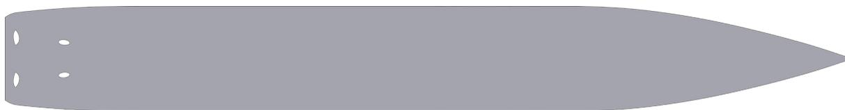
Figure 11.2 Waterplane area at draft of 8.2 m from the NAPA model of the cruise ship
