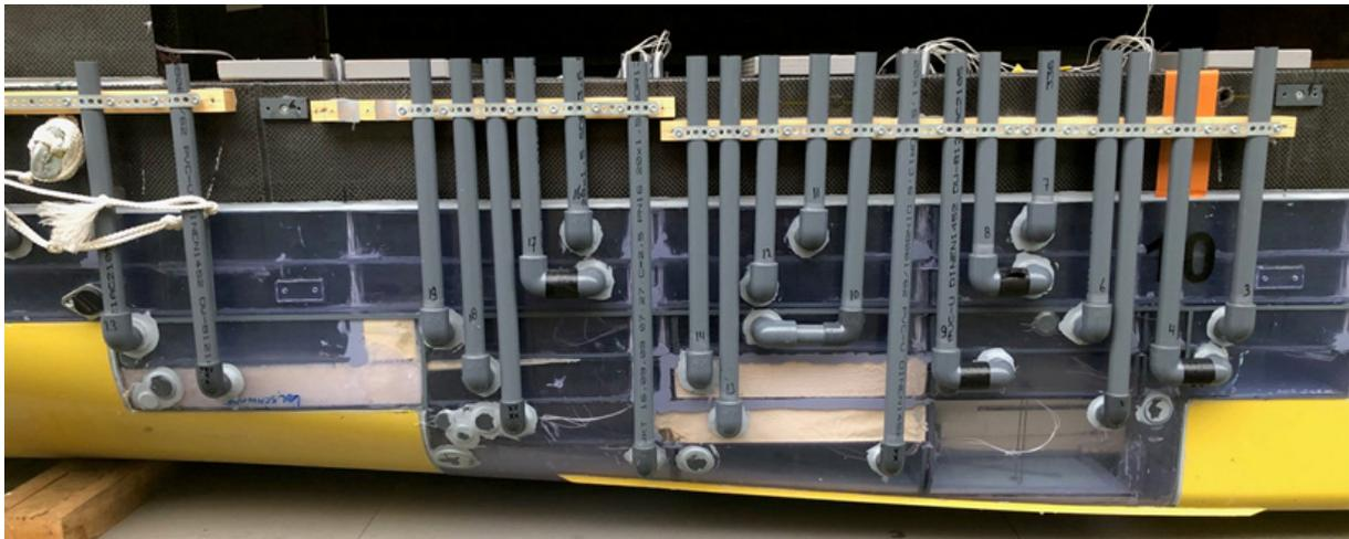
Figure 6.36 Air pipes in the model for ventilating the flooded compartments (courtesy of MARIN)
