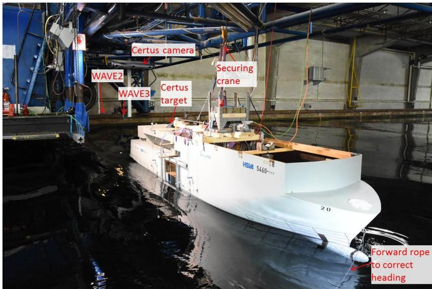
Figure 7.6 Test setup for transient flooding (courtesy of HSVA)
