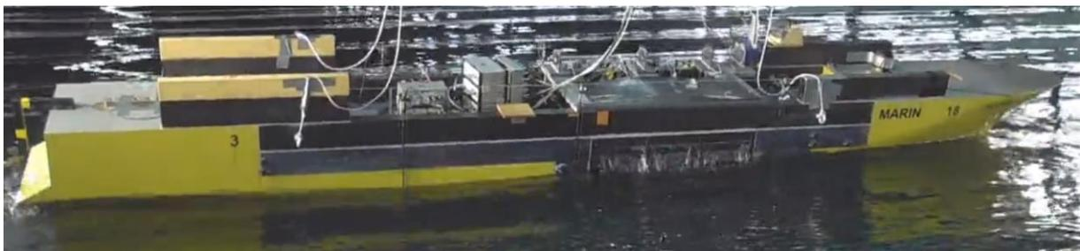
Figure 6.17 Cruise ship model in irregular beam seas (courtesy of MARIN)
