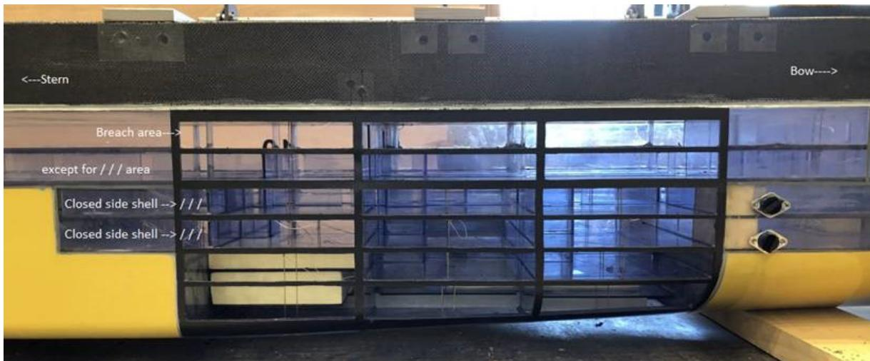
Figure 6.3 Breach opening in the SB side of the model (courtesy of MARIN), note that on decks 3 and 4 the breach length is smaller in the aft end
