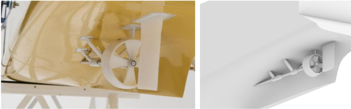
Figure 6.8 Appendages of the cruise ship model (photo courtesy of MARIN)
