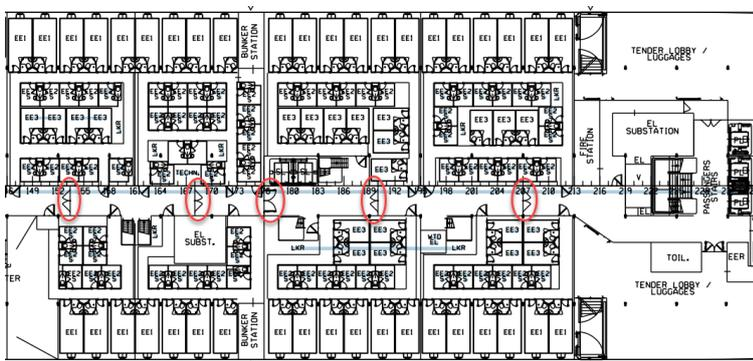
Figure 5.18 Initial general arrangement of the deck section, with planned double leaf doors in the service corridor (Courtesy of Chantiers de l'Atlantique)
