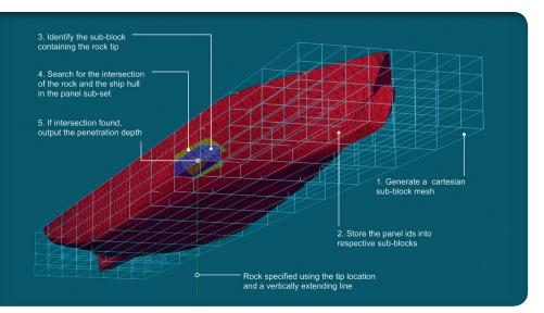
The purpose of this workspace is to combine ship navigation risk models with methods combining computational structural dynamics and evasive ship hydrodynamics to better understand the cause and effect of accidents on crashworthiness and hence widen the scope of flooding management. risk Multimethods with physics variable configuration and complexity make use of state-of-the-art knowledge.
